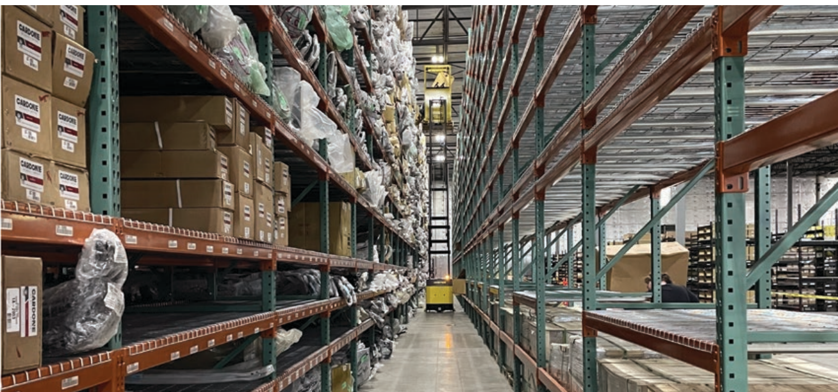
Conventional racking with wire security guidance for forklifts (notice grooves in the floor)
