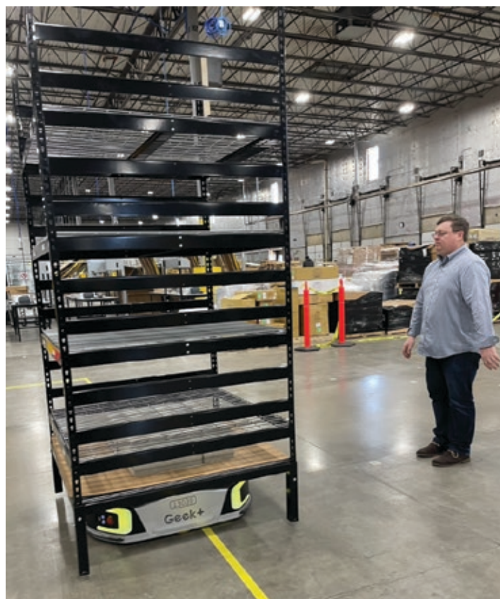
Demonstration of safety features of Geek+ robots, which can detect nearby objects and slow down to avoid collisions
