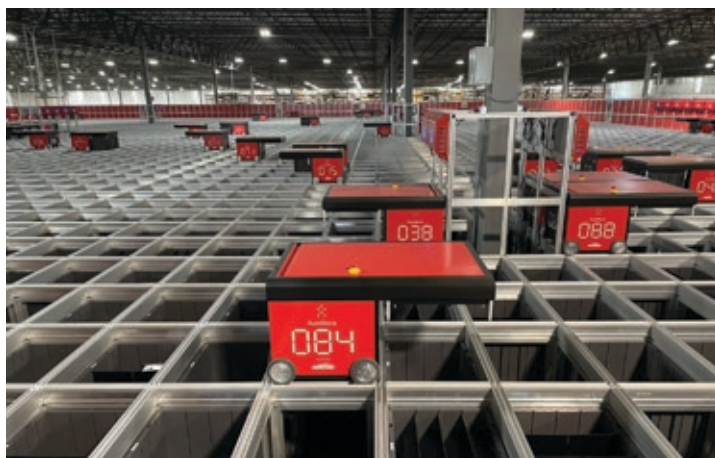
Top of AutoStore system with its robots
